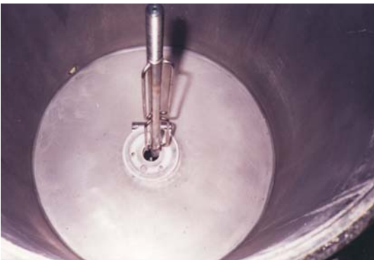
Figure 6. - PRK Center Post/Sealing Plate Installed
