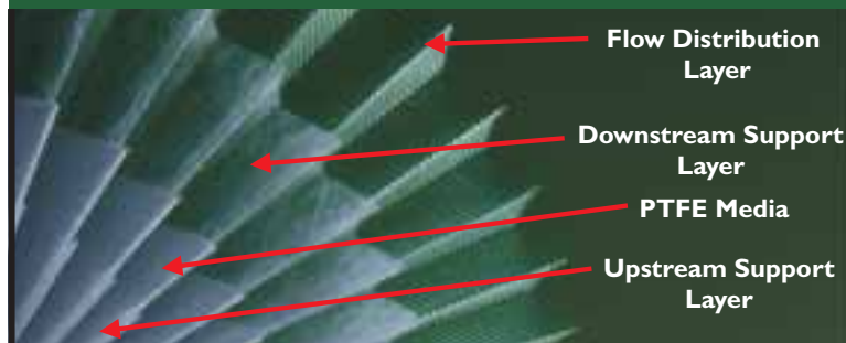
Photo 2. - Microfluo ® r II Filter Construction
