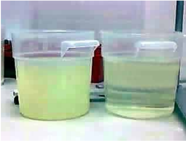
Figure 5. Turbidity improvement made with 3M Purification filtration system. Before 3M Purification filtration, left, and after 3M Purification filtration, right
