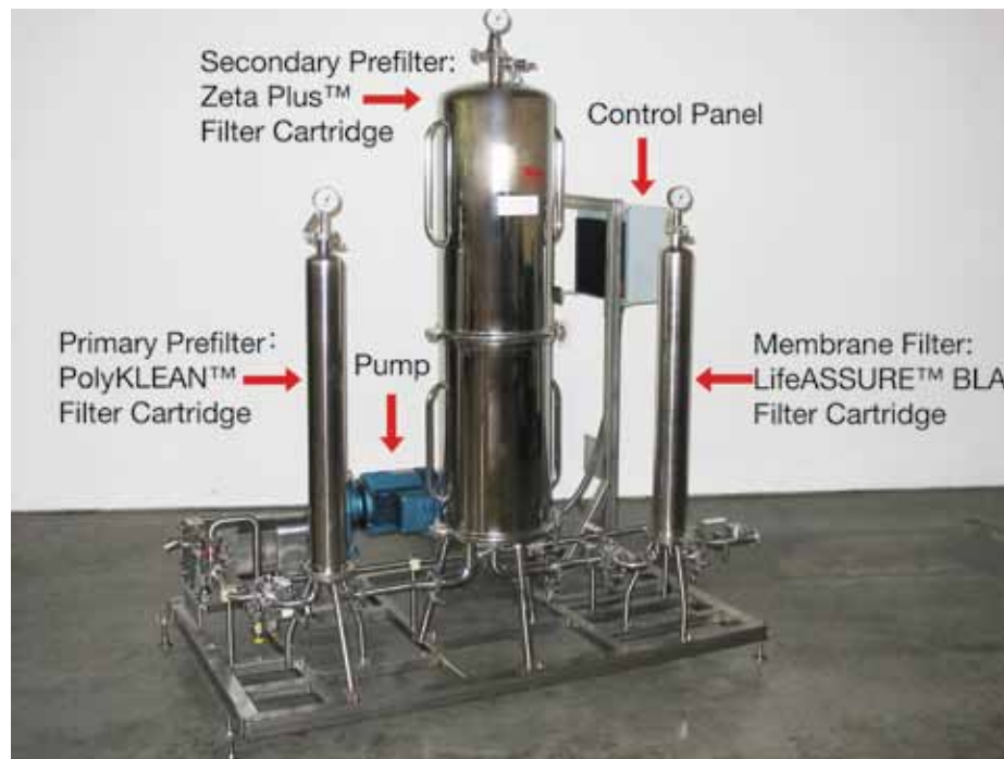
Figure 9. Three-stage filtration system for anti-browning solution
